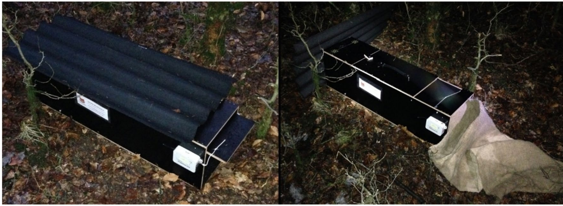
Fig. 1 Wooden box traps with electronic trap sensor system
